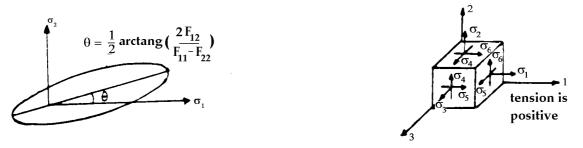
Figure 2.1. Failure ellipsoid and definition of positive stresses.
